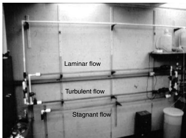
**Figure 1** This plumbing model system was designed to study the effect of flow regimes on *Legionella* presence within biofilm. The test section consisted of three parallel clear PVC sampling pipes (from top to bottom: laminar, turbulent and stagnant) of 1 inch in diameter. The four transition ports (4 inch diameter) were connected to inlets and outlets of laminar and turbulent flow sampling pipes to create smooth entry and exit conditions.
