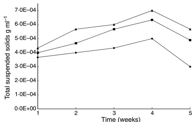
**Figure 3** Comparison of total suspended solids (TSS) in inlet biofilm samples ( $Re\ 1 = 355$ ,  $Re\ 2 = 34\ 825$ ). More TSS were recovered from the biofilm of the turbulent flow pipe than that from the laminar flow pipe, while the lowest amount was recovered from the stagnant flow pipe. Legends: ▲, Turbulent flow; ■, Laminar flow; ●, Stagnant flow.
