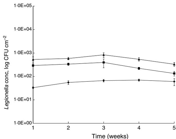
**Figure 2** Comparison of *Legionella* concentration in inlet biofilm samples ( $Re_1 = 355$ ,  $Re_2 = 34\ 825$ ). Significantly higher number of *Legionella* counts were recovered from the biofilm of turbulent flow pipe than that from the laminar flow pipe, while the lowest counts were recovered from the stagnant flow pipe ( $P = 0.01$ ). Legends: ▲, Turbulent flow; ■, Laminar flow; ●, Stagnant flow.
