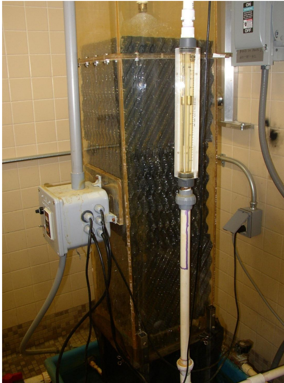
Figure E21 – T1 (Control) prior to PEFD (Trial 2/2). Packing has been replaced and seasoned
