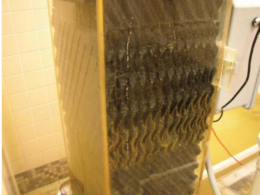
Figure F25 – Close-up of T2 (Device) packing prior to ED trial.
