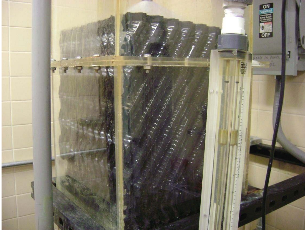
Figure G22 – Close-up of T1 packing prior to UD trial
