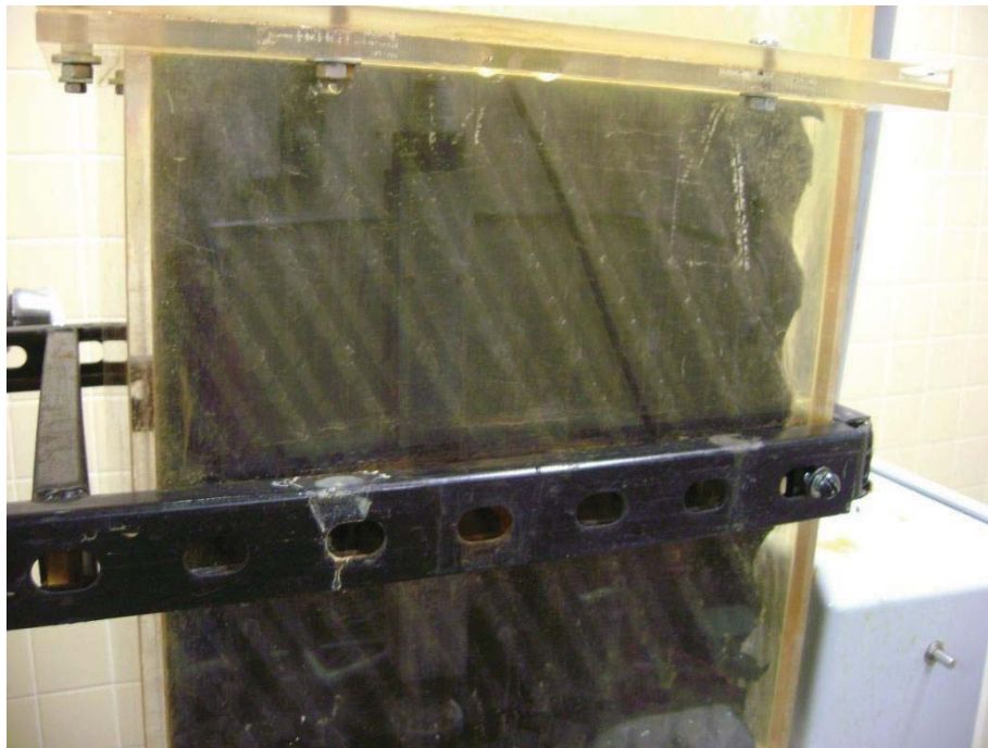
Figure G26 – Close-up of T2 (Device) packing prior to UD trial
