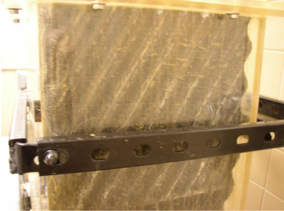
Figure E27 – Close-up of T2 (Device) packing following PEFD (Trial 2/2)
