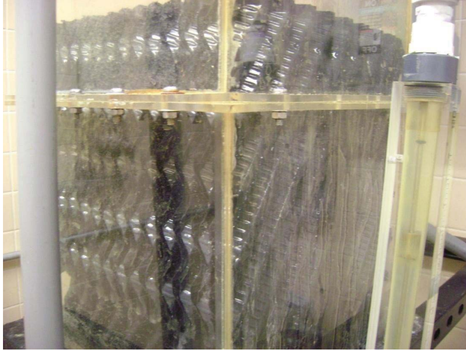
Figure G28 – Close-up of T1 (Control) packing following UD trial
