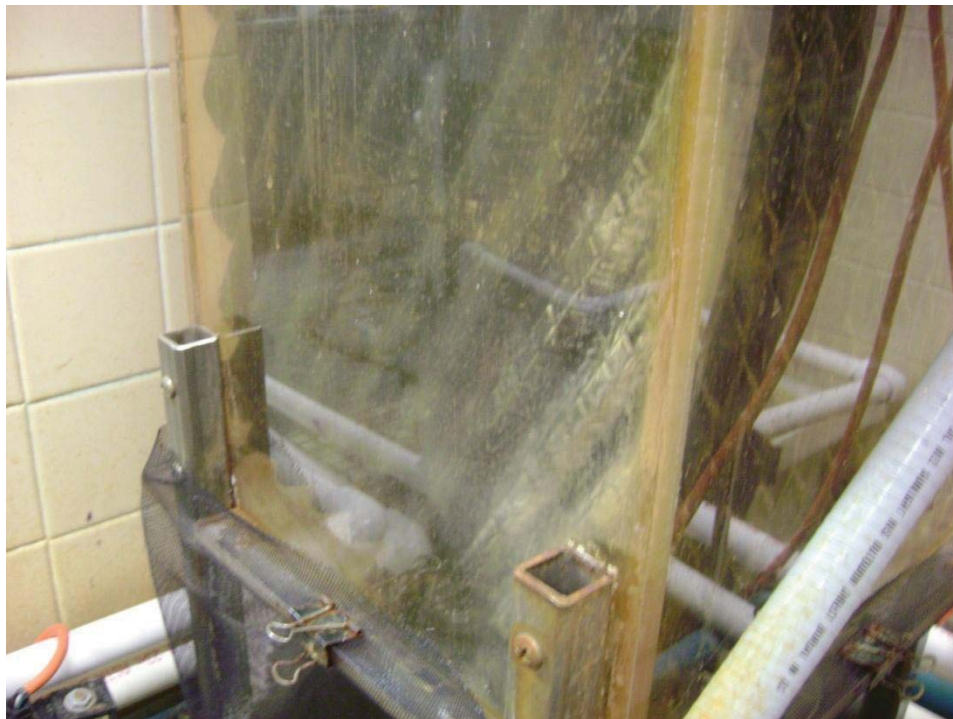
Figure G32 – Close-up of T2 (Device) packing following UD trial
