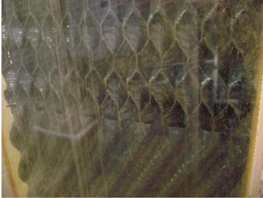
Figure G25 – Close-up of T2 (Device) packing prior to ultrasonic treatment device trial
