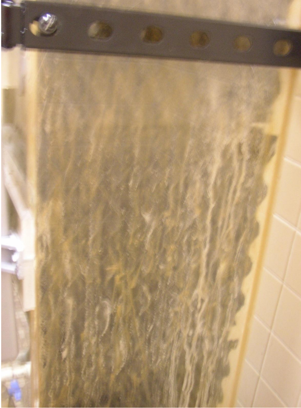
Figure D27 – Close-up of Tower 2 packing after PEFD Trial 1/2
