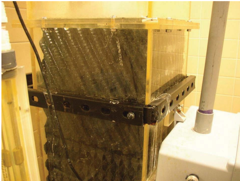
Figure F26 – Close-up of T2 (Device) packing prior to ED trial
