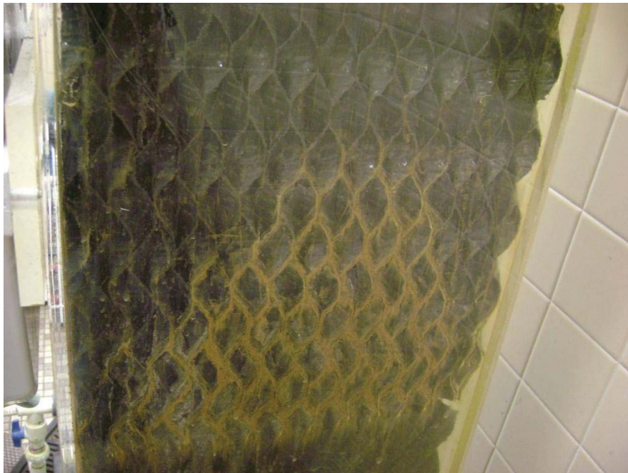
Figure F31 – Close-up of T2 (Device) packing after ED trial
