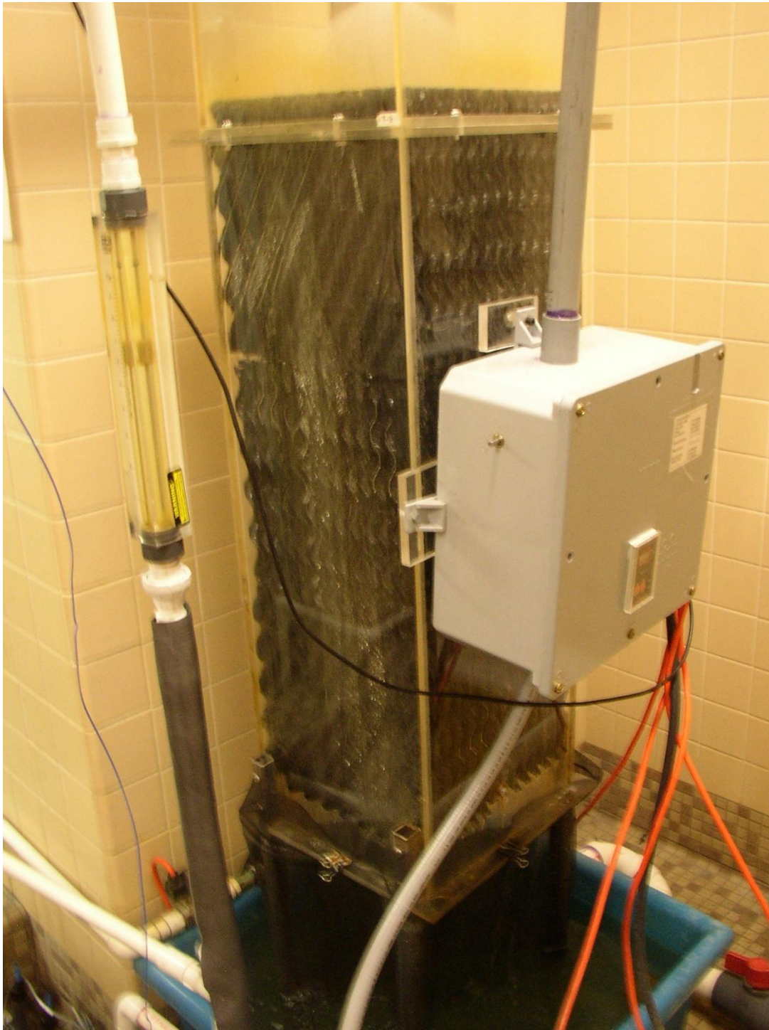
Figure C22 - T2 (Device) prior to MD trial. Packing has been replaced and seasoned. *Note device placement on tower entrance stream. Device has been protected with a shield of lead to eliminate electrical interference.
