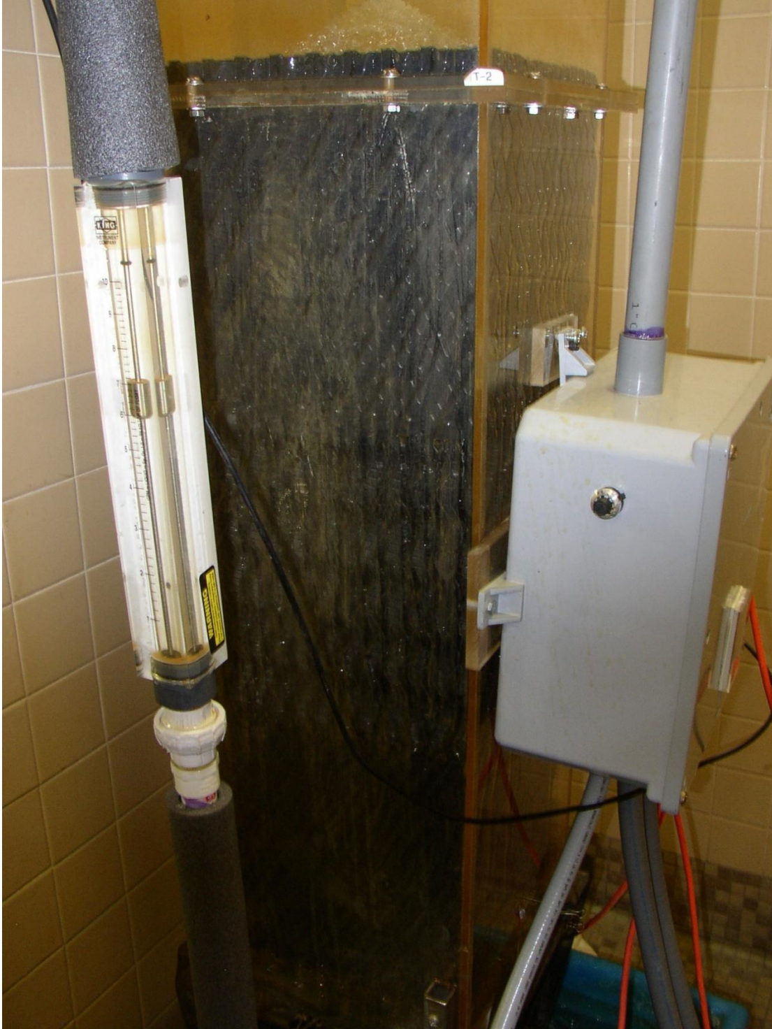
Figure D22 – T2 (Device) prior to PEFD Trial 1/2. Packing has been replaced and seasoned
