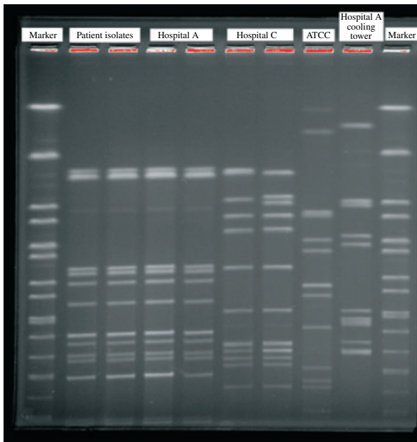
FIG. 1. The pulsed-field gel electrophoresis pattern showed that the Legionella pneumophila serogroup 3 of the patient matched the L. pneumophila serogroup 3 from hospital A, but not hospital C. ATCC, American Type Culture Collection.
