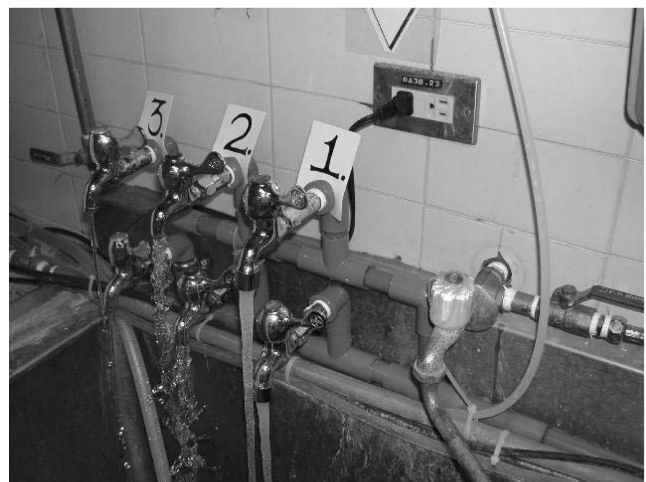
FIGURE. Experimental set up of the model plumbing system (1, faucets with aerators; 2, control faucets; 3, faucets with laminar water flow devices).
