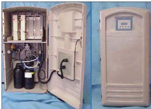
The chlorine dioxide ( $\text{ClO}_2$ ) generators (above) in this study use an electrical source and membrane technology to produce  $\text{ClO}_2$  from a sodium chlorite precursor. The membranes are housed in removable cassettes in the upper portion of the unit (left). The generators eliminate the need for handling hazardous chlorine gas or strong acids.
